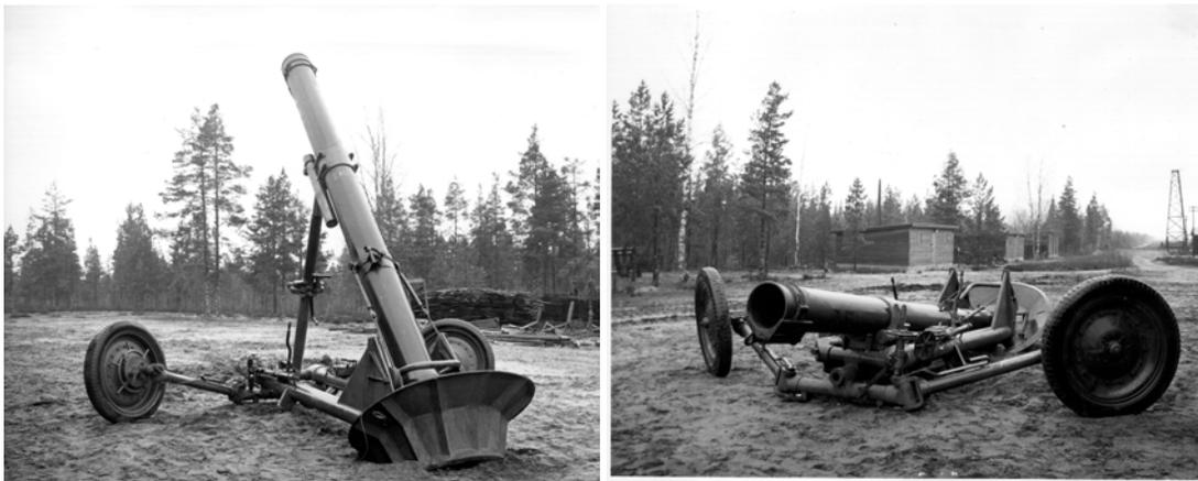
FIGURE 2 300 Krh/42 in firing position and with barrel lowered for loading [1]
