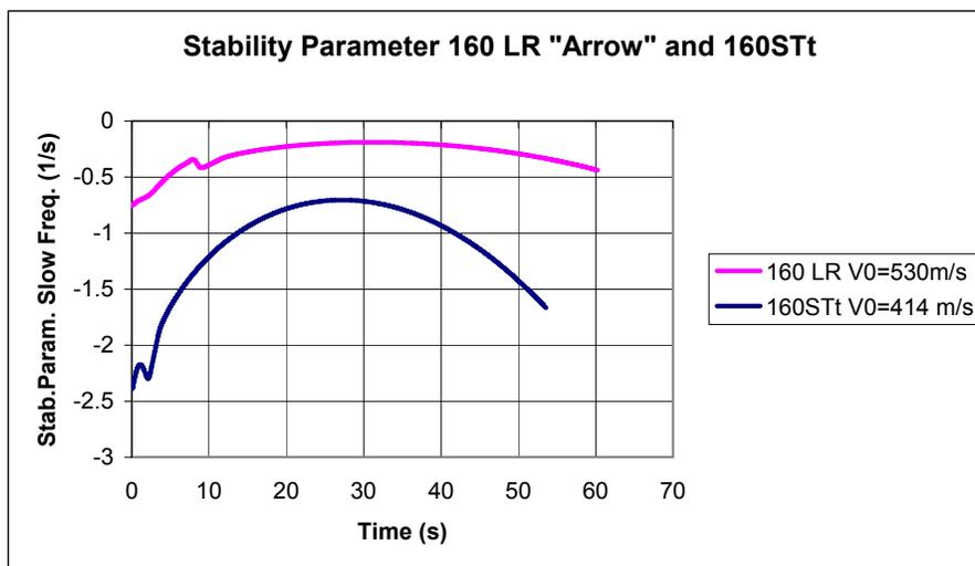
FIGURE 10 Dynamic stability of 160 STt and 160LR arrow projectiles
